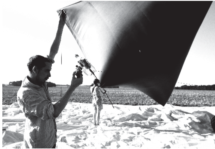
Aerocene Gemini travels 605 km distance, floats over 12 hours, reaches 16,283 m altitude. All without any carbon, fossil fuels, helium, hydrogen, burners, or engines—using only air currents and the heat of the sun. 2016. Courtesy Aerocene Foundation. Foto/Photo: Studio Tomás Saraceno.
